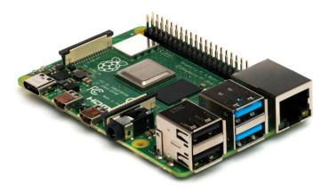
**Processor** 4-core CPU, clock speed 1.5GHz
